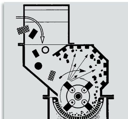
principle hammer impact mill
