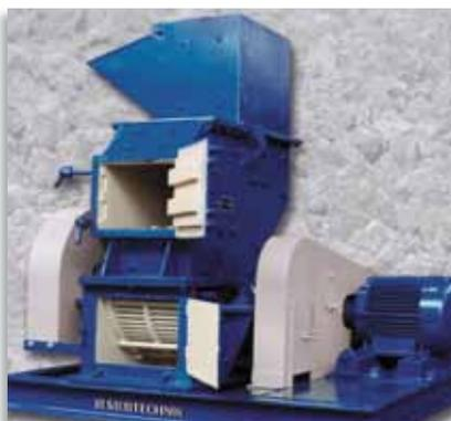
hammer impact mill HPM 3 with feed hopper
